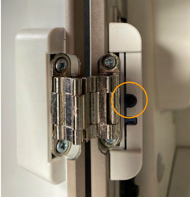
Microswitch on the hinge of the rear cabinet door
