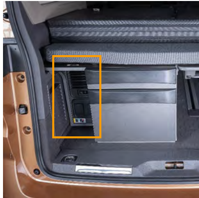
Equipment box on the left-hand side of the vehicle at the rear
