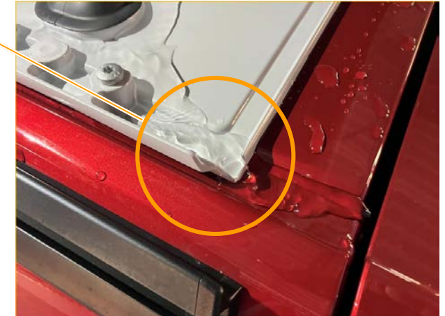
Rear water drain on the roof cross member
