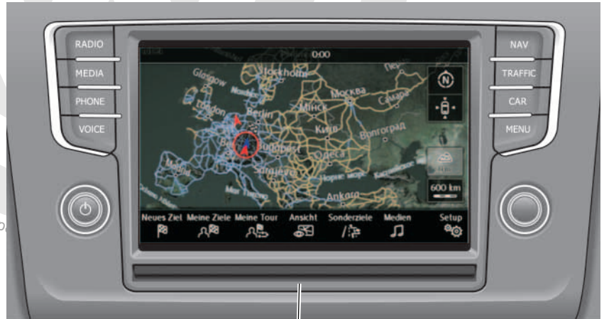
Infrared proximity sensor behind the operating and display unit panel
