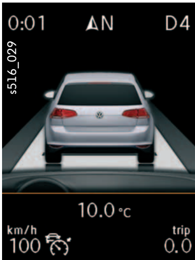
Distance control – small actual distance, large target distance
