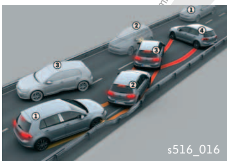
Accident situation without multicollision brake
