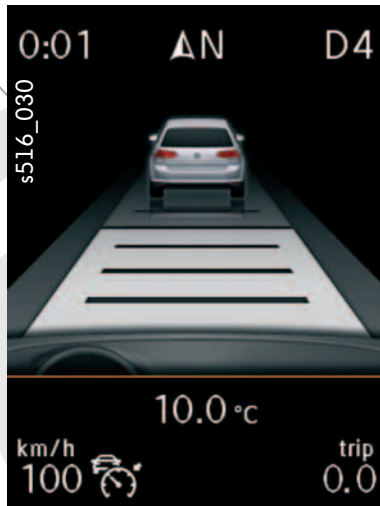
Distance control – large actual distance, large target distance (TI 4)
