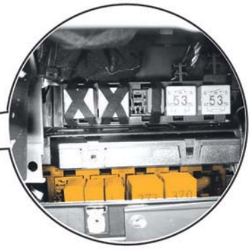
Relay carrier underneath onboard supply control unit
