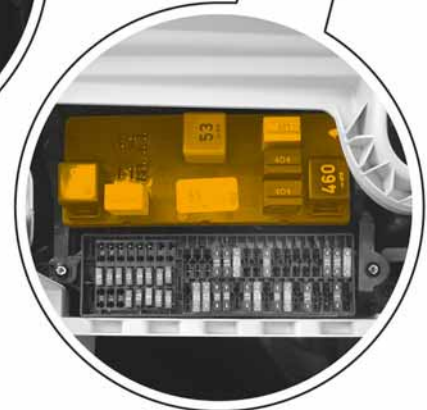
Relay carrier on onboard supply control unit, under dash panel on left
