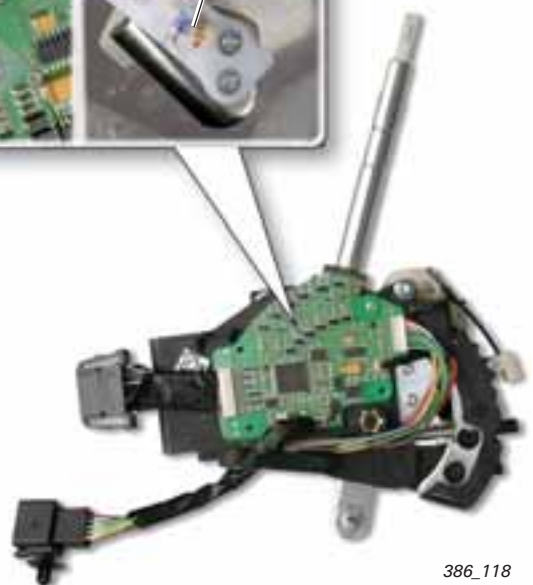
Hall sensors for the determination of selector lever positions P, R, N, D and S Protected by copyright permitted unless a with respect to tl
